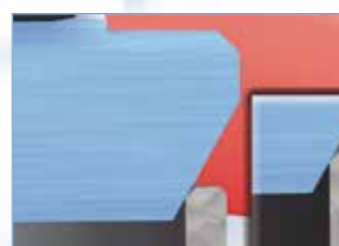
"Cut-off effect" – the conical shape of the marginal seat causes surface deposits to be removed during sealing.
