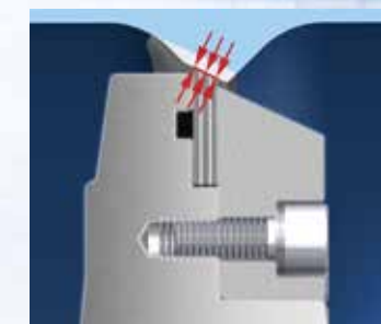
The ZETRIX® process valve seals according to the area seating principle; the required contact pressure is applied via the actuator, which can be switched off as a function of the torque.
