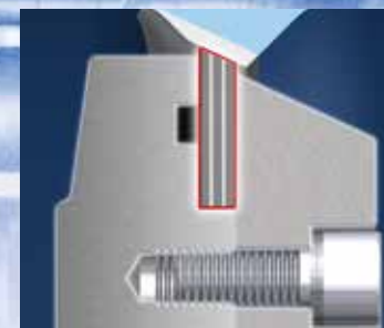
Lamellar structure made of stainless steel and graphite lends additional elasticity to the sealing ring. Double sealing mechanism in the form of a special, spiral-wound gasket made from a heat-resistant elastic material.
